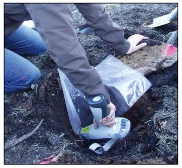
Figure 16. XRF measuring in small trial pit at Stångberget. Photo: S. Dahlin 140410.
