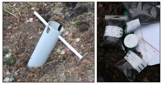
Figure 13. Humus drill for soil sampling. The drill Figure 14. Collecting of soil samples. consists of a steel serrated plastic tube, which is rotated down into the soil and pulled up with the soil core. Photo: H. Almqvist 100505.
